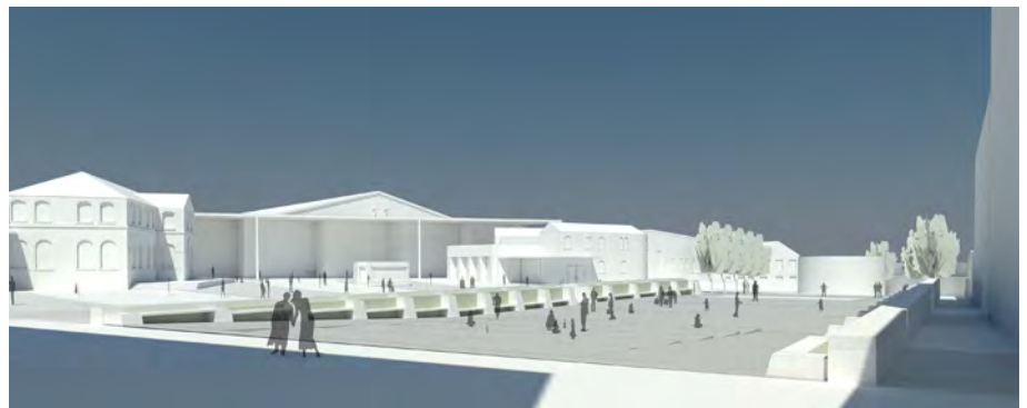
Fig.104 View C : Entry to the Coal Drops from the south is to be provided with steps and 1:20 grade ramps
