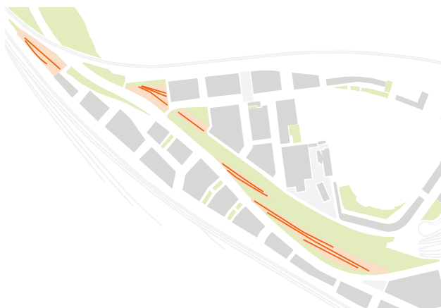
Fig.79 Areas of railway tracks to be retained and where applicable, filled with ballast and planted
